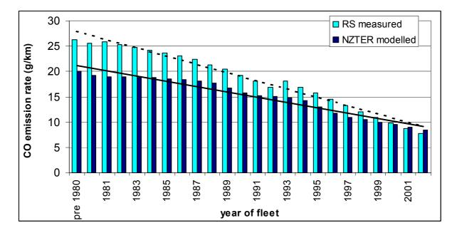
Figure 1 Comparison of modelled and measured CO emission rates for petrol cars
