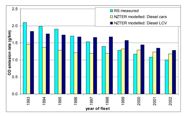
Figure 5 Comparison of NZTER modelled diesel car and light commercial vehicles CO emissions with RSD measurements
