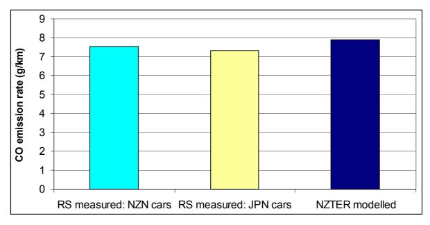
Figure 4 Comparison of modelled and measured New Zealand new (NZN) and Japanese used (JPN) CO emissions for petrol cars for fleet year 2002
