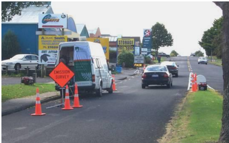
Figure 2 The remote sensing system in action with the on-road display showing a "fair" reading in the background.
