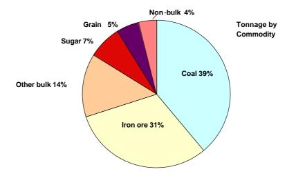
Bulk rail freight principally comprises coal (39% of tonnes carried) and iron ore (31% of tonnes carried). Other bulk commodities hauled include forest products, ores and minerals, cement, limestone and petroleum products.
