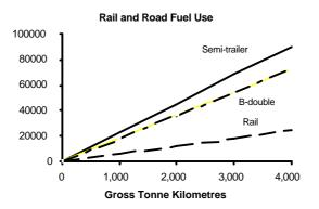
Melbourne replaces 150 semi-trailers and saves over 45,000 litres and 130 tonnes less of greenhouse gas emissions of fuel compared to road transport including road pickup and delivery.<sup>2</sup>
