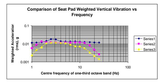
Figure 2 Comparison of seat pad weighted vertical vibration versus frequency
