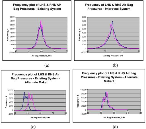
Figure 1 Comparison of Air Bag Frequency Histograms – (a) Existing System (b) Improved System, (c) Existing System - Alternative Make, (d) Existing System -Alternative Make 2
