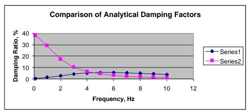
Figure 3 Comparison of predicted orifice controlled damping (Series 1) and capillary controlled damping (Series 2)
