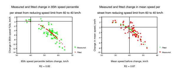
Figure 2. Measured and fitted changes in speed parameters on 60® 40 streets (a) 85th percentile speeds (b) mean speeds
