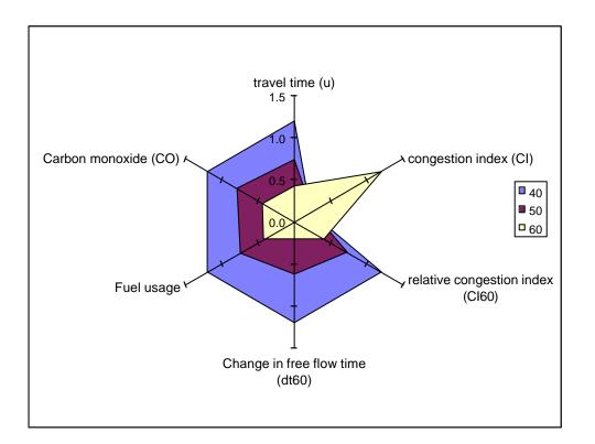
Figure 1. Starplot of modelled traffic performance indicators for different speed limits (60, 50 and 40 km/h) for test network C [source: Taylor (2000)] [The arms of the star represent the relative performance of a network under 40, 50 and 60 km/h speed limits on the six performance indicators of travel time, congestion index, relative congestion index (60 km/h datum), change in free flow travel time, fuel consumption and CO emissions]
