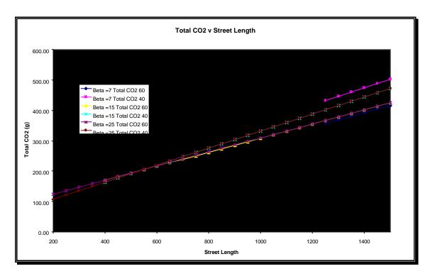
Figure 4. Total CO<sub>2</sub> emissions and street length, showing crossover effect at 550 m
