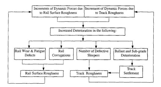
Figure 2 Interactions of deterioration of track components
