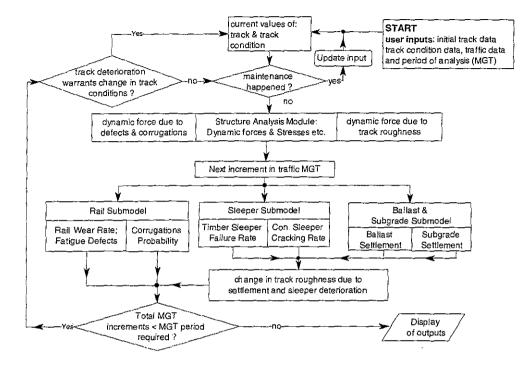
Figure 1 Framework of integrated model
