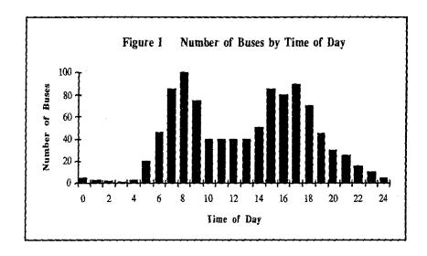
Figure I shows the varying fleet requirements for the "Newtown" depot throughout the entire day. For ease of calculation it is assumed that the depot has these fleet requirements 5 days per week for 50 weeks of the year and in every hour of operation the buses all operate at the same speed. With this assumption and the information contained both in Figure I and Table III the results of following three approaches of allocating the unit cost per vehicle are outlined
