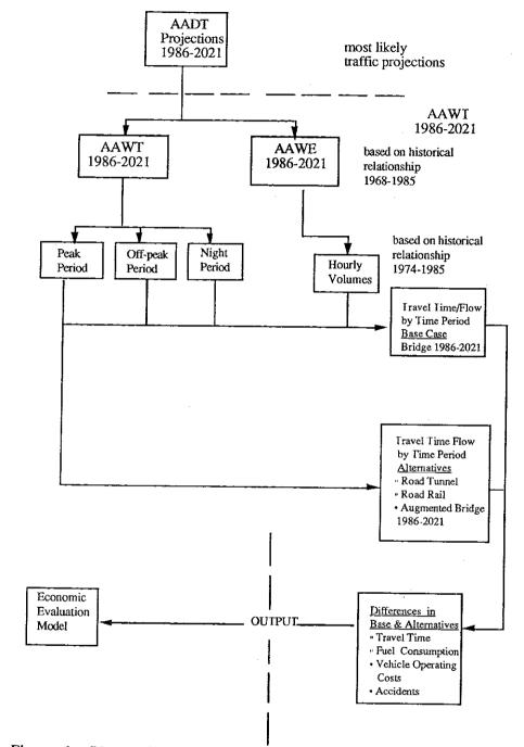
Figure 1. Flow diagram of traffic forecasting methodology and economic evaluation model for Sydney cross-harbour transport
