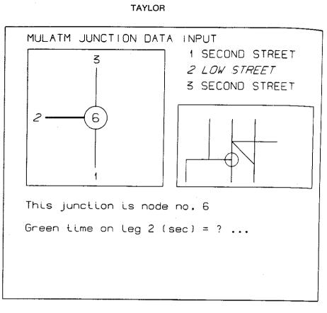
Figure 1. Junction Data Input in MULATM using Interactive Graphics
