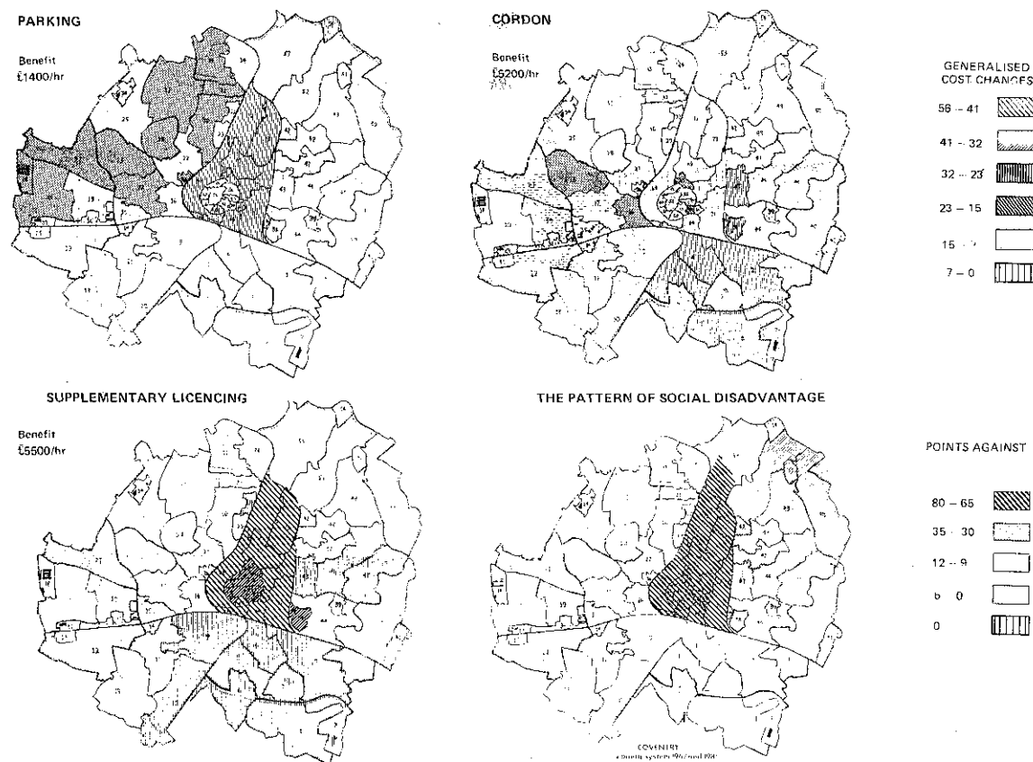
FIG. 4 Accessibility Variations for Otherwise Comparable Policies (Coventry) After (Wigan et al. 1974)
